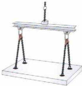
1. Spreader beam as above.
